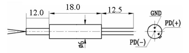
Standard Package for Infrared Band. For other wavelength band, size may vary due to special detector configurations.
